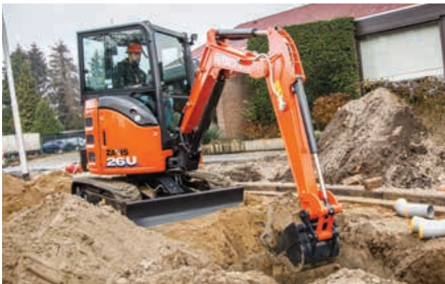
The front of the machine is fitted with a boom cylinder guard for added durability.
