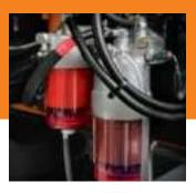
■ Engine oil, fuel and hydraulic pilot oil filters are all located on the same side at ground level for easy servicing.
