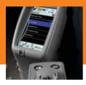
■ Multi-language LCD monitor and rotary dial provide intuitive access to machine info and functions. Just turn and tap to select work modes, monitor maintenance intervals, check diagnostic codes and set cab temperature. Control oil flow and toggle between dig and thumb modes with a programmable thumbattachment mode.
