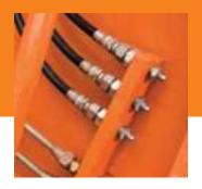
Centralized lube banks place zerks within easy reach, making greasing less messy and timeconsuming.
