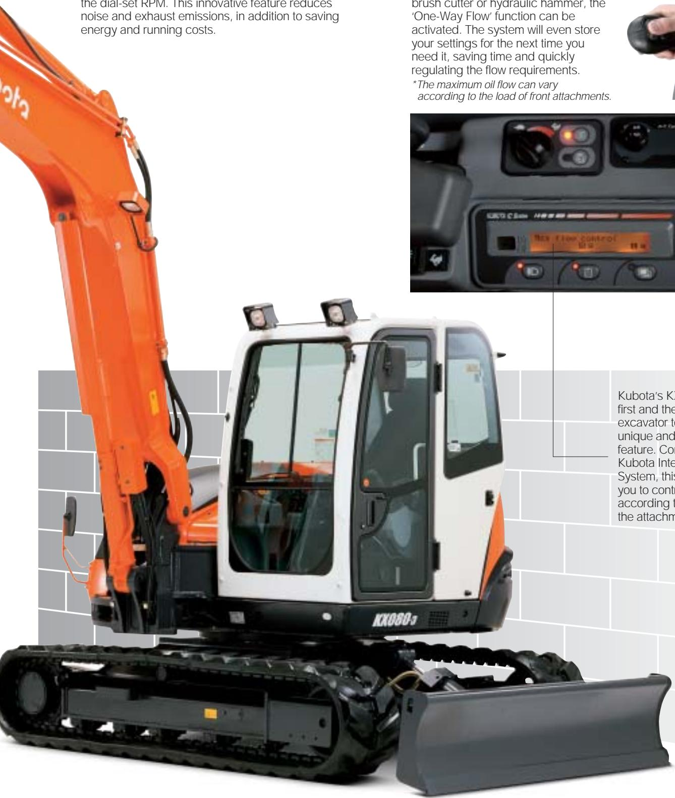
Kubota's KX080-3 is the first and the only mini/midi excavator to offer this unique and revolutionary feature. Combined with the Kubota Intelligent Control System, this function allows you to control the oil flow according to your needs or the attachment in use.
