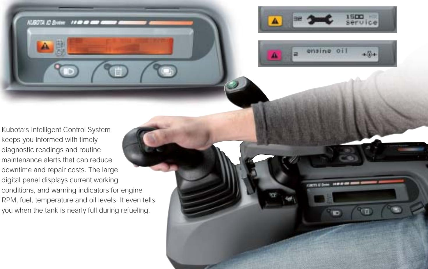
Kubota's Intelligent Control System keeps you informed with timely diagnostic readings and routine maintenance alerts that can reduce downtime and repair costs. The large digital panel displays current working conditions, and warning indicators for engine RPM, fuel, temperature and oil levels. It even tells you when the tank is nearly full during refueling.
