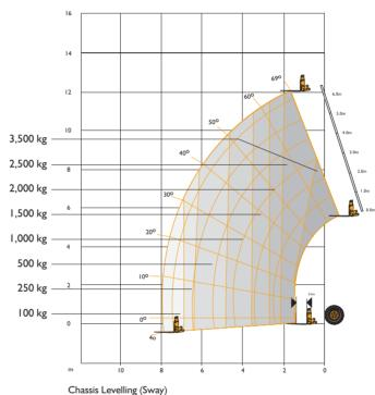
With stabilisers retracted (Sway angle  $\pm 9^{\circ}$ )
