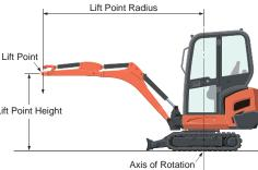
\*The lifting capacities are based on ISO 10567 and do not exceed 75% of the static tilt load of the machine or 87% \*\*The excavator bucket, hook, sling and other lifting accessories are not included on this table.
