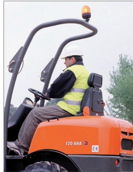
Driving site with folding FOPS structure
