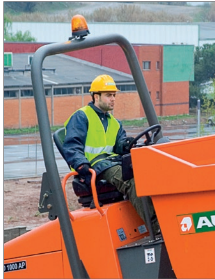
Driving site with folding FOPS structure
