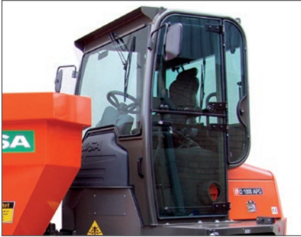
Sound-proof and ROPS/FOPS closed cabin (D 150/175 R, D 201 R & D 600/1000 A)
