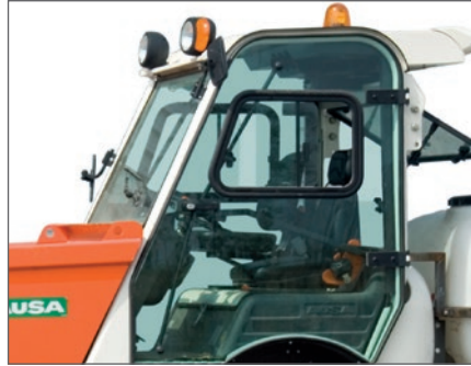
Sound-proof and ROPS/FOPS closed cabin (D 150/175 R, D 201 R & D 600/1000 A)
